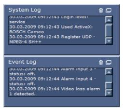
The **System Log** field contains information about the operating status of the VideoJet X10 and the connection. You can save these messages automatically in a file (see *Section 5.15 Advanced Mode: LIVEPAGE Functions, page 43*).
